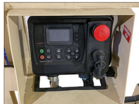
Weatherproof Ignition Panel
