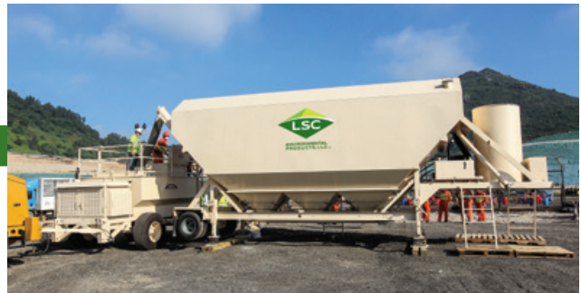
Horizontal silo loading powdered product into a Posi-Shell® Applicator.
